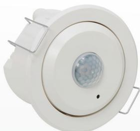
The MD-O is an intelligent, fully digital presence detector for office lighting. The sensor excels with its speed: MD-O reacts to a unique combination of motion and sound. The light is switched on immediately as soon as someone enters an office and stays on while someone is working quietly. If a radio is left on after working hours, then the lighting will be switched off.
